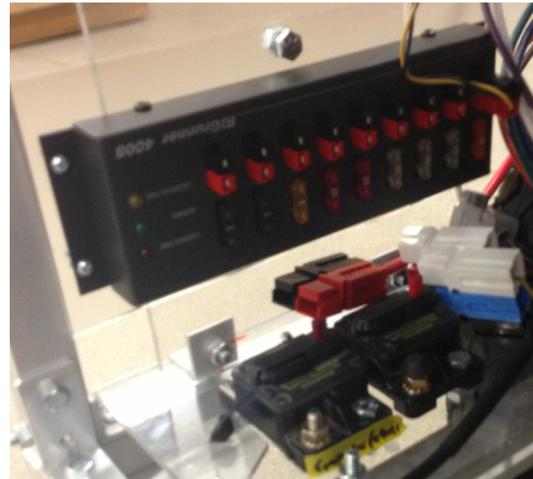
Figure 4. **Demonstrating the serviceability aspects for ease-of-use operations.** The figure on the left shows the battery compartment tray sliding out of the robot for easier serviceability. The figure on the right shows the breakers of the motor controller and the power distribution (PD) board that routes power to all the sensors.
