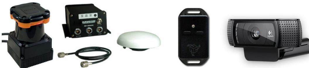
Figure 10. **The main sensors used to provide feedback and perception of the world to the robot.** The sensors are, from left to right, the Hokuyo LIDAR, the NAVCOM GPS, the IMU, and the Logitech webcam.
