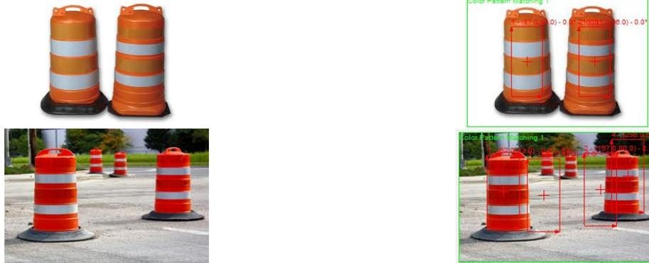
Figure 15. **Results of some barrel detection via color classification.** The top row shows the ideal case with the barrels being correctly classified due their features, sizes, pattern, and contrast. The bottom row shows a more realistic case where although the barrels were detected, the algorithm also detected some noise.
